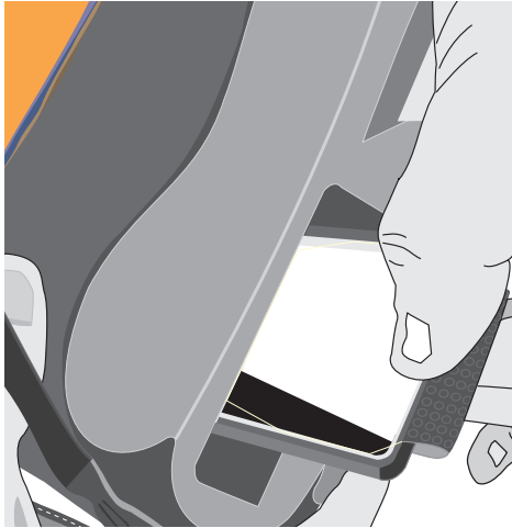
Figure 3.4: PCMCIA card removal
