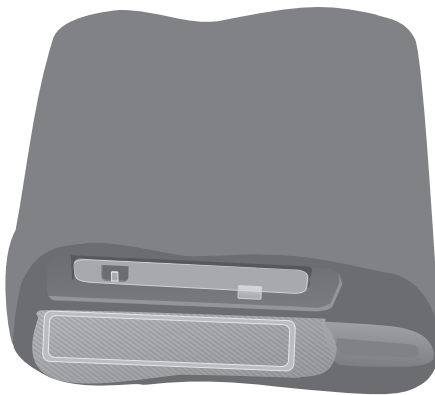
Figure 3.9: Opening Battery Bay Door
