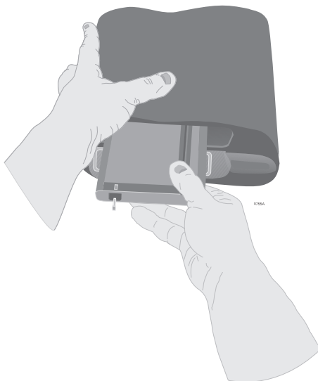
Figure 3.13: Removing Battery From Receiver (B)
